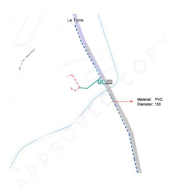
RELOCATION OF PIPELINE Maharlika Highway, La Torre L = 630 m
